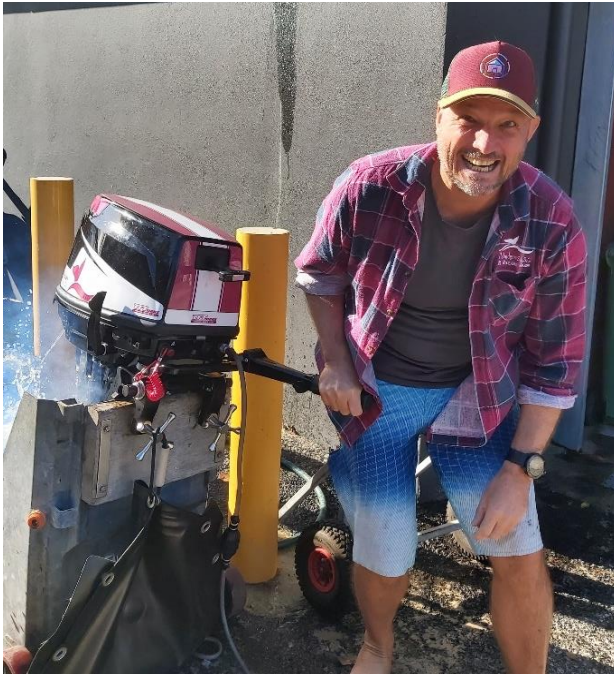
Did you know it takes 10 hours to “run in” a new IRB motor? Pictured here is Kyal Thornton putting in his time to make sure the new motor is ready to go. IRBs are the key piece of rescue gear, but do require constant maintenance and attention. Behind the scenes, people like Kyal make a key, often unacknowledged, contribution to the Club’s ability to provide lifesaving services.
